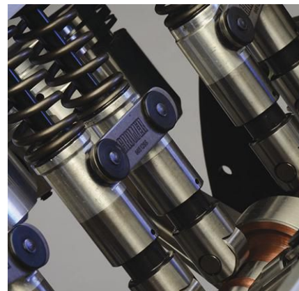
Today's roller cams/lifters allow for more aggressive cam profiles. (Photo courtesy Crower)
