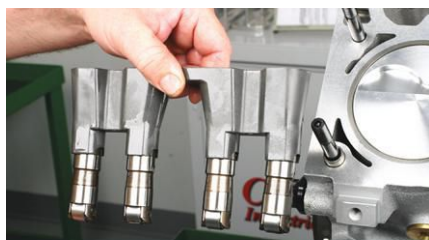
A group of LS lifters secured in a lifter tray. The flats on the lifter bodies align with female flats in the tray.
