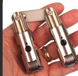
The location of oil feed holes on hydraulic and solid lifter bodies must align with the oil galleries within the lifter bore to ensure adequate oil delivery.
