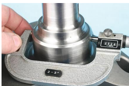
All main journals measured spot-on at 2.749 inches. With standard main bearings, the oil clearance is 0.003-inch.
