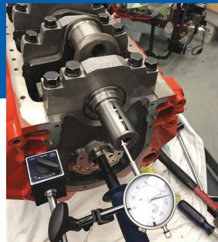
After installing all main caps to fully seated positions, all bolts were loosened, and the crank was knocked fore/aft to aid in centering cap alignment.
