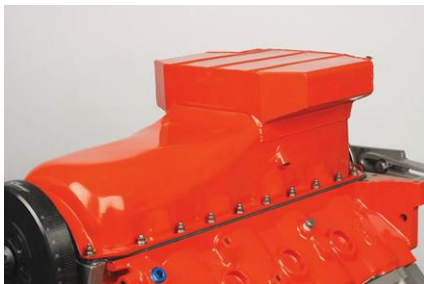
The Moroso oil pan was secured with a one-piece Moroso gasket and an oil pan stud kit from ARP.
