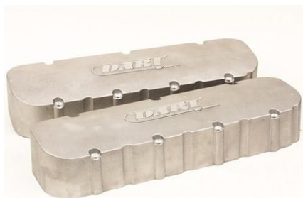
The Dart cast aluminum valve covers feature an inverted flange design, providing added clearance for rockers and an optional stud girdle.
