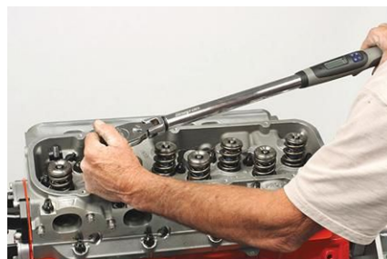
All ARP head stud nuts were torqued to 70 pound-feet, following the standard big-block Chevy sequence.
