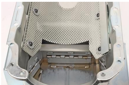
A view of the sump baffles. The one-way, lightly spring-loaded baffle doors keep oil from leaving the sump area.
