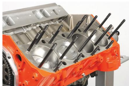
Head studs were installed during test-fitting. All holes are blind, but lower threads were lightly coated with high-friction lube to avoid future sticking.
