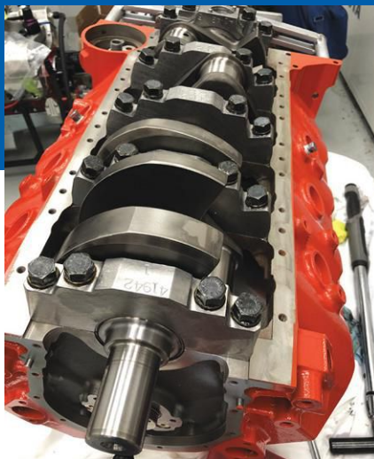
All main cap bolts were torqued in several steps.
