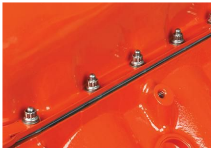
We secured the oil pan with ARP stainless studs and 12-point nuts, using stainless mil-spec flat washers between the nuts and the painted surfaces.
