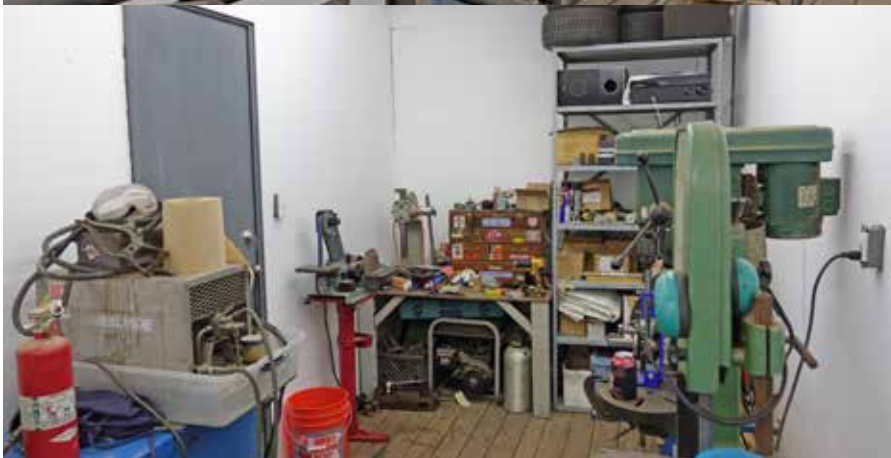
King found his high-cube, 9-foot-tall aluminum container locally in Apple Valley, California. He's outfitted it with lighting, air conditioning, a man door and a hoist to lift the engine in and out of the race car.
