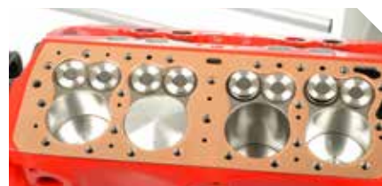
Copper head gaskets are a popular choice for many flathead builds.
