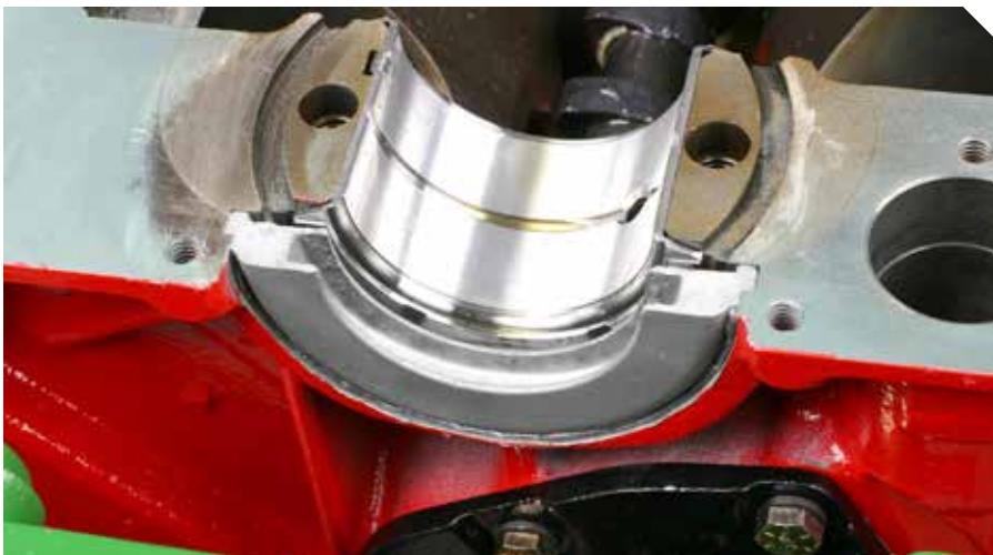
Original rear main rope-type seals can be troublesome to install to seal properly. New braided graphite rope seals tend to work much better.
