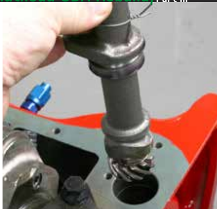
Apply high-pressure lube to the oil pump gears before meshing with the cam-driven intermediate gear.
