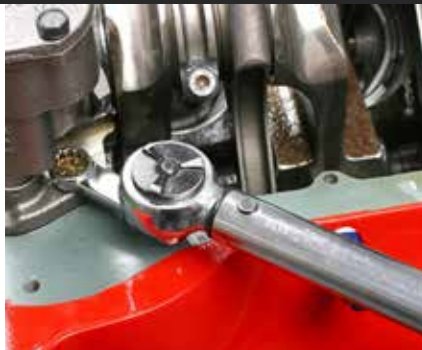
Because of limited access to the oil pump mounting bolt, a 2-inch torque wrench extension was required. To achieve the spec 15 pound-feet, when using the 2-inch extension on a 14.5-inch torque wrench, I set the torque at 13.5 pound-feet.
