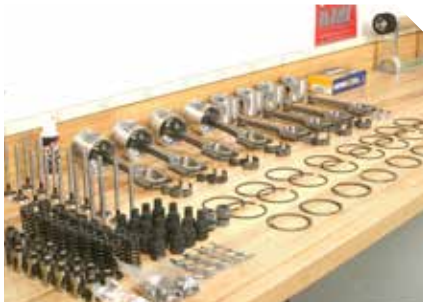
Prior to final assembly, all components were detail-cleaned and organized. All rings were file-fit for each dedicated cylinder.
