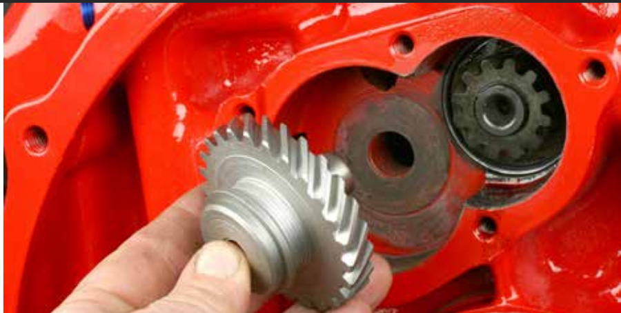
With the cam already installed, the oil pump gear is inserted with its guide into the hole, then rotated to engage cam-to-gear mesh. Apply assembly lube to the gears prior to installation.
