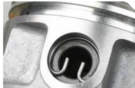
The pistons we used feature full-float wrist pins. C-clips are installed to retain the pins. Installation is easy with needle-nose pliers.
