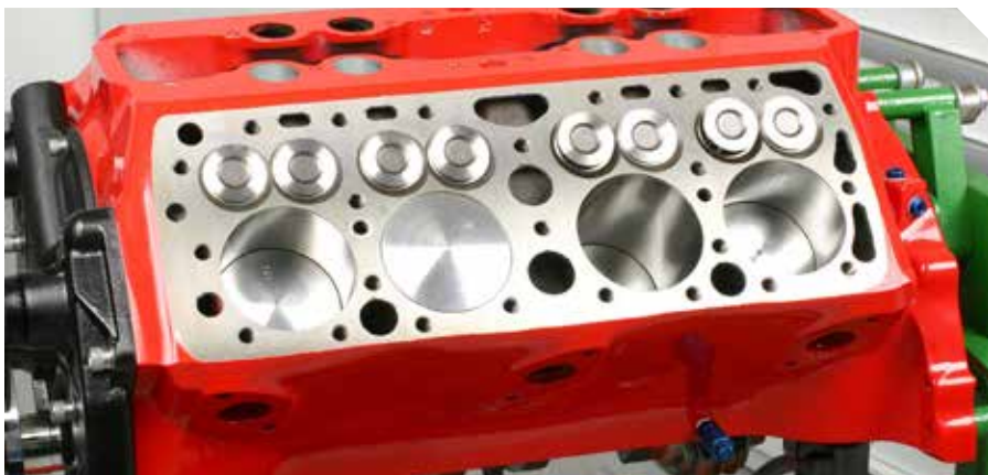
With valves and pistons installed, decks were carefully cleaned of any oil prior to cylinder head installation. All head bolt holes were cleaned using a dedicated thread chase during initial block prep.
