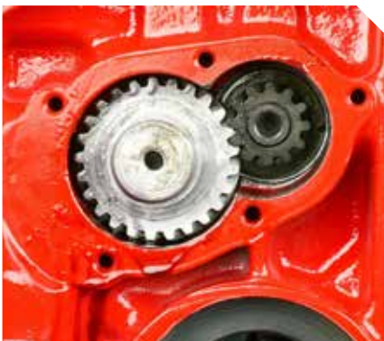
The oil pump gear fully installed.
