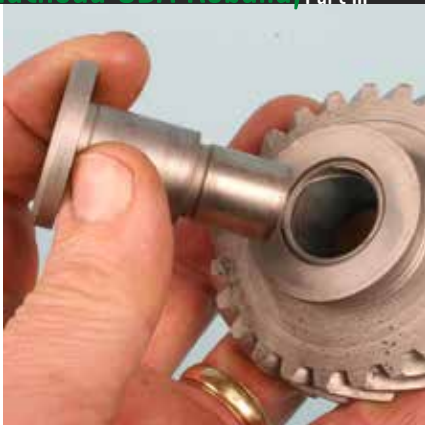
The oil pump drive gear features a steel guide that registers into a locating hole in the rear of the block.
