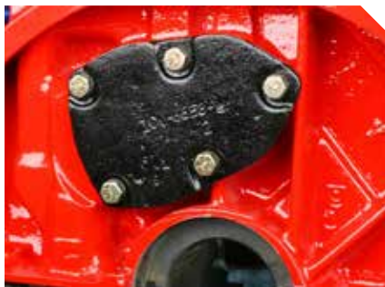
A cast iron cover plate (with gasket) seals off the rear oil pump gear and cam. This is one of the parts that you need to save from the old engine core.
