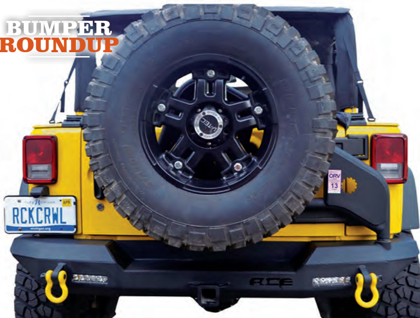
Remember that aftermarket rear bumpers and/or tire carriers can add weight to the rear of the vehicle. (Photo courtesy ACE Engineering and Fab)
