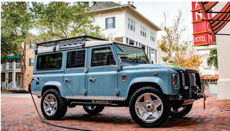
Project Britton features a Heritage-style grille, swing-away wheel carrier, sidesteps with SVX silver inserts, Front Runner roof rack and ladder, sand beige Porsche Nappa leather, Recaro Expert S seats, a classic Evander Wood wheel, and teak wood flooring and teak wood bench. (Photo courtesy E.C.D.)
