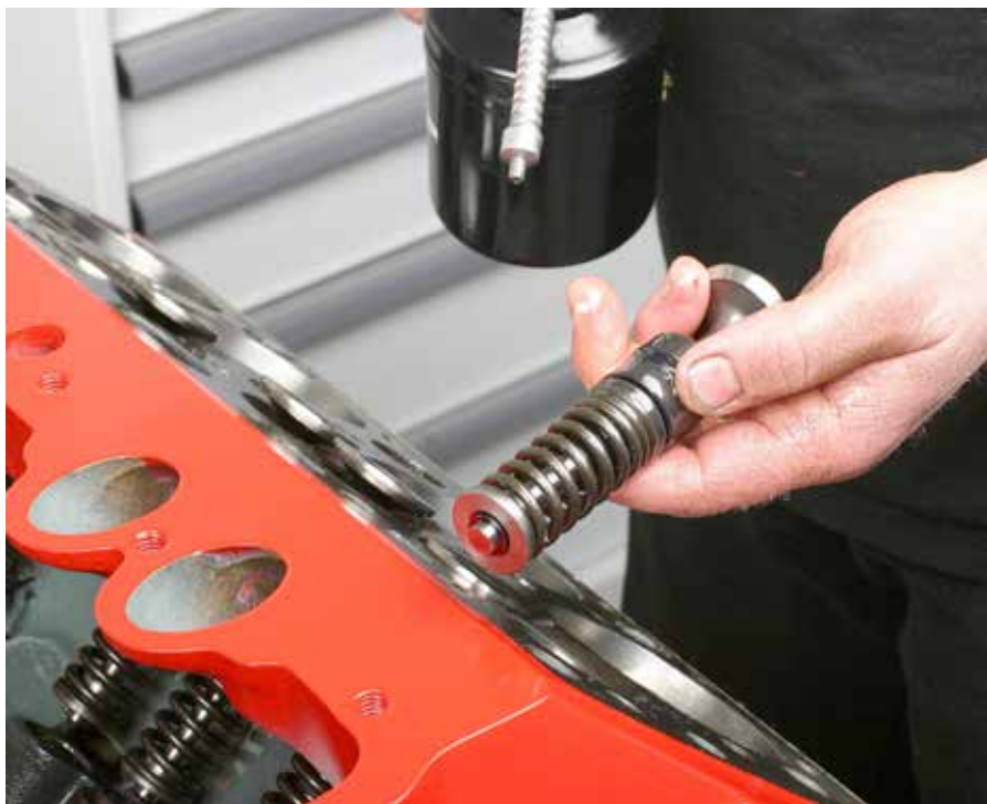
The flathead design features valves in the block. Lube the assembly prior to insertion.
