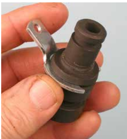
Once the valve assembly is inserted into the block, a retainer clip installs from inside the lifter valley to a groove in the valve guide. This keeps the valve captured in the block. A flathead-style manual valve spring compressor tool is used to compress the spring to allow installation of the clip.
