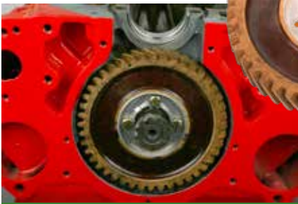
The cam gear installed with locking tabs to prevent bolt loosening. I also applied a dot of medium-strength threadlocker to the bolt threads.
