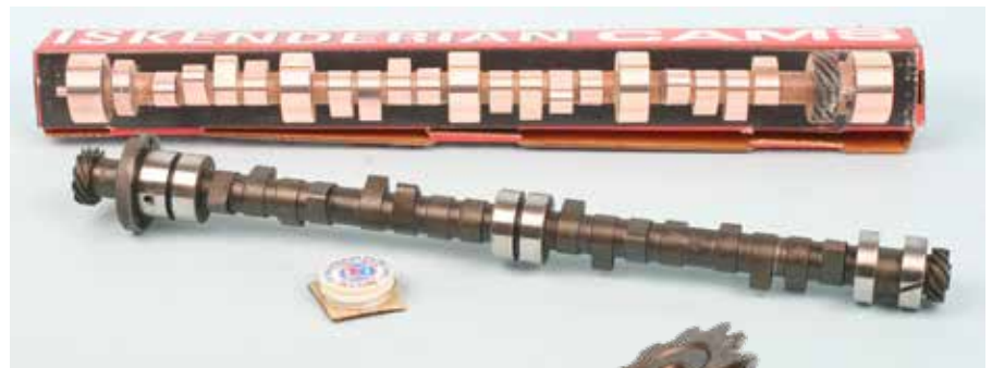
Our ISKY flat-tappet cam features a valve lift of 0.320" at intake and exhaust, 264 degrees duration intake/exhaust, and a lobe center of 108 degrees. Valve lash is set at 0.012" cold and 0.010" hot.
