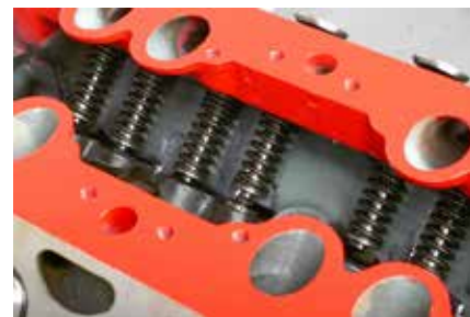
Lifters are lubed and installed into their bores prior to inserting the valves.
