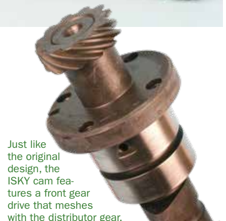
Our ISKY flat-tappet cam features a valve lift of 0.320" at intake and exhaust, 264 degrees duration intake/exhaust, and a lobe center of 108 degrees. Valve lash is set at 0.012" cold and 0.010" hot.
