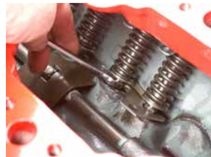
To adjust the valves, rotate the hex-headed adjusters. To prevent the lifters from rotating (adjuster-to-lifter threads are very tight), a special bracket holds a pair of lifters in place during the adjustment process.
