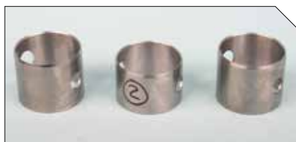
Per the flathead design, three cam bearings are required. The center bearing is noticeably shorter.
