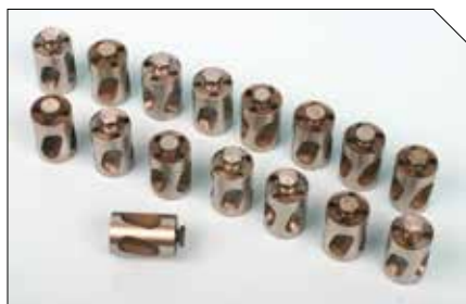
New flat-tappet solid lifters feature interference-fit threads to hold valve adjustment.
