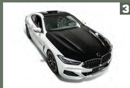
1. Installing PPF such as Avery Dennison Supreme Defense gloss paint protection film protects vehicles from dings, dents, road debris, insects and weather. Quality films are self-healing and provide a sleek, gloss finish. 2. PPF appeals to high-end vehicle clients. 3. A pigment-rich black paint protection film provides protective accents and contrasting effects. This BMW showcases Avery Dennison neo noir PPF.
