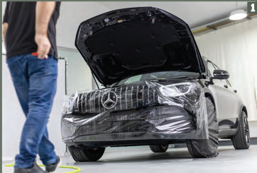
1. Installing PPF such as Avery Dennison Supreme Defense gloss paint protection film protects vehicles from dings, dents, road debris, insects and weather. Quality films are self-healing and provide a sleek, gloss finish. 2. PPF appeals to high-end vehicle clients. 3. A pigment-rich black paint protection film provides protective accents and contrasting effects. This BMW showcases Avery Dennison neo noir PPF.
