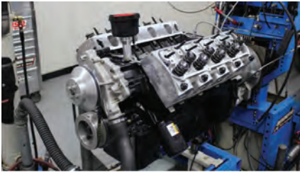
An efficient head with better low- and mid-lift flow numbers usually shows its stuff up top. (Photos courtesy AFR – Air Flow Research)
