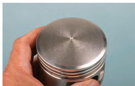
The finished dome shape was changed from an original radius of 5.304 inches to a "softer" radius of 6.985 inches. With a 0.057-inch-thick head gasket, we have a piston-to-chamber clearance of 0.057-inch.
