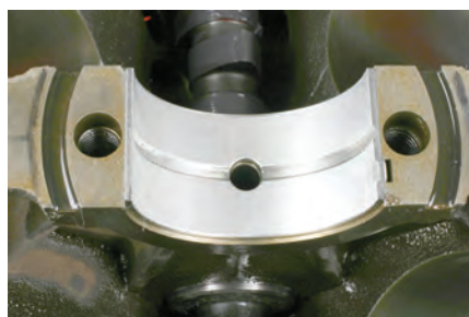
Note that the main block saddles feature curved grooves at each side, which register the main caps. However, there's a bit of play, so the caps must be tightened gradually in stages.
