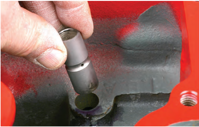
The original bushing installs to the block.
