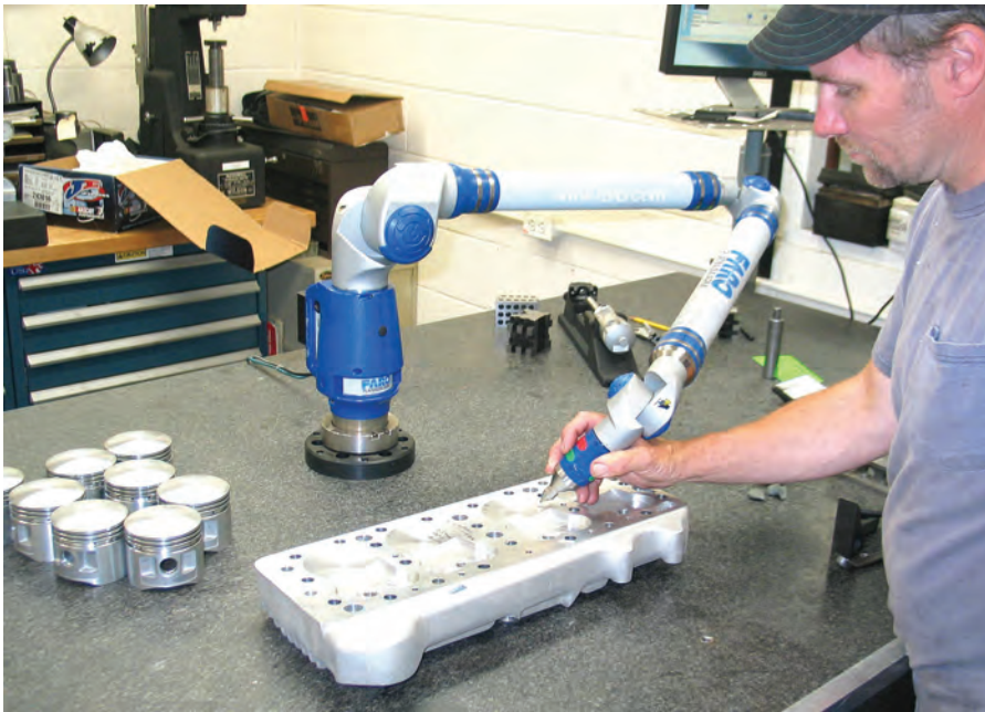
Due to our piston dome radius, our increased stroke and the 65cc chambers, things got a little tight. We had the piston domes re-contoured at G.L. Heller. Here, a technician measures and plots the chamber shape using a CMM coordinate probe.
