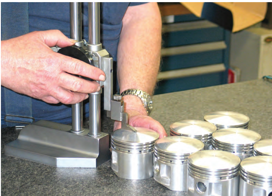
Piston dome height was also measured. The combined data was then uploaded to a CNC lathe, where each piston dome was lightly radiused to meet our required clearance.
