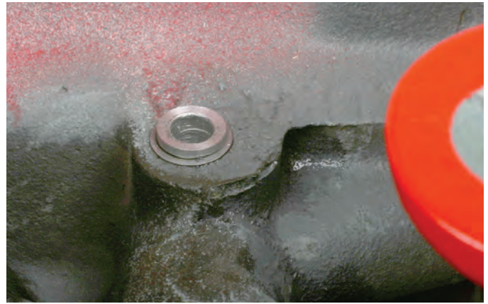
The aluminum bushing liner is installed.
